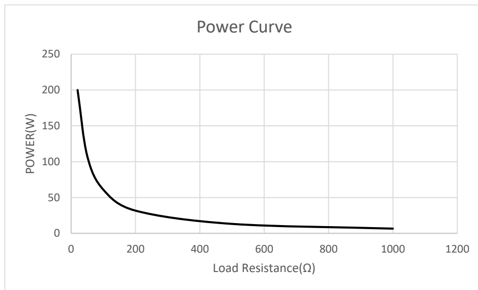
Figure 5 Diagram of output power versus impedance
